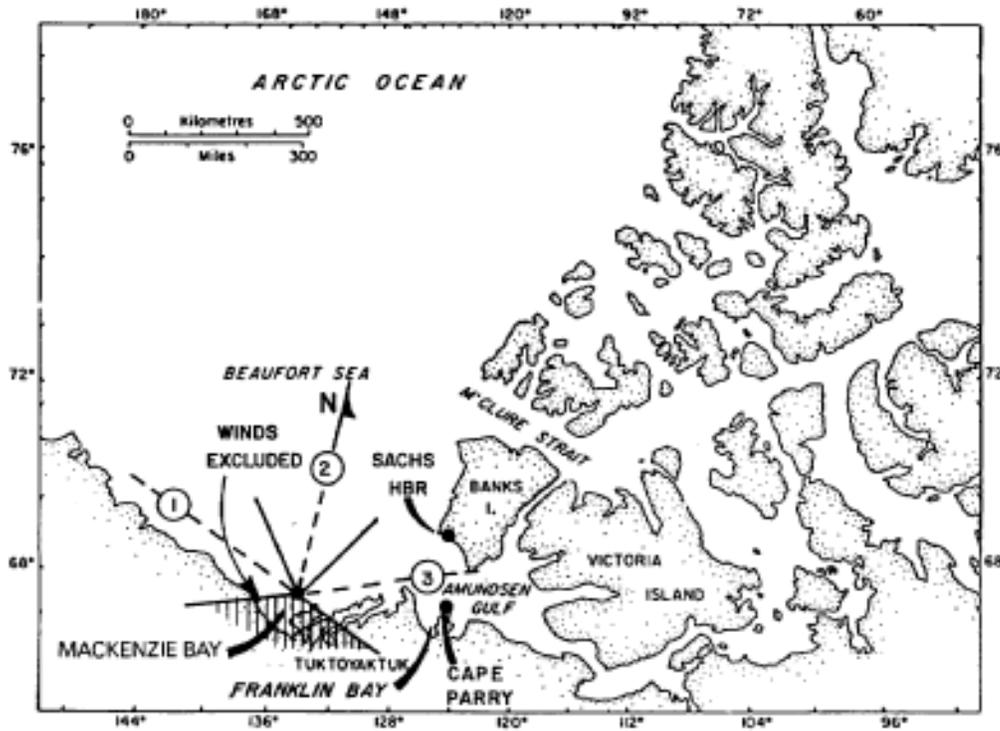
Figure 2.7 Wind measurement stations and the storm class breakdown used by Dames & Moore - 1975.
